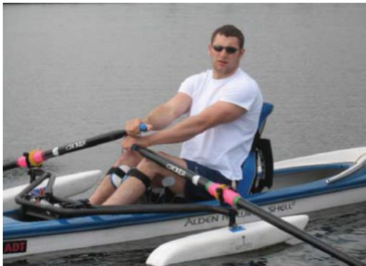
Figure 99: The Alden 16 (single) recreational boat adapted for FES
