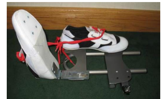
Figure 40: Modified foot stretcher with retaining screws with soleplate removed and heel hinged.
