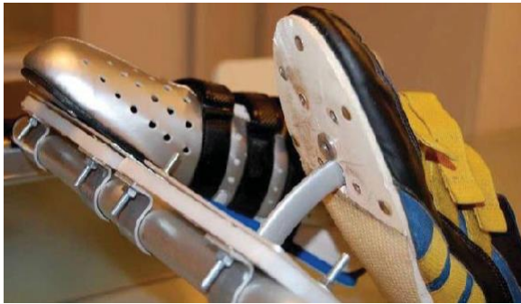
Figure 41: Shimano foot stretcher for rower with Arthrodesis (Fused ankle joint)
