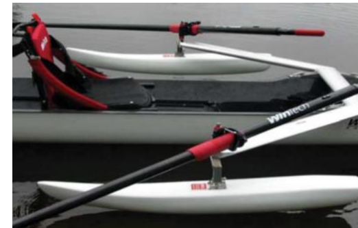
Figure 20: A single scull (1x) with stabilising pontoons
