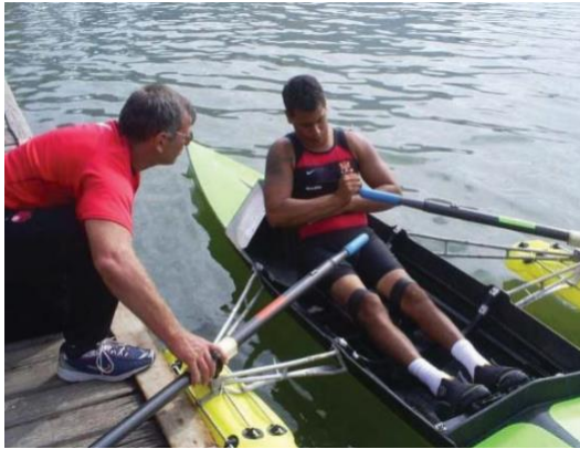
Figure 34: Buoyancy bags modified as pontoon floats
