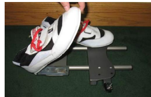
Figure 40: Modified foot stretcher with retaining screws with soleplate removed and heel hinged.
