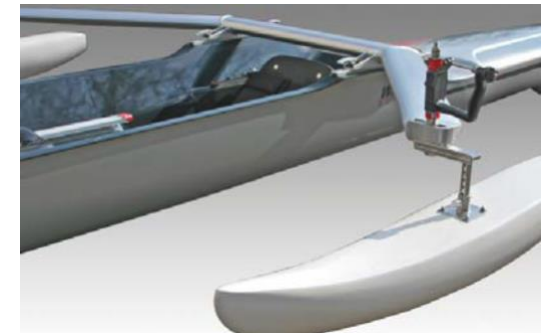
Figure 20: A single scull (1x) with stabilising pontoons
